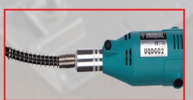
Pass collet cap through inner spring of flexible shaft and insert inner spring in the collet
