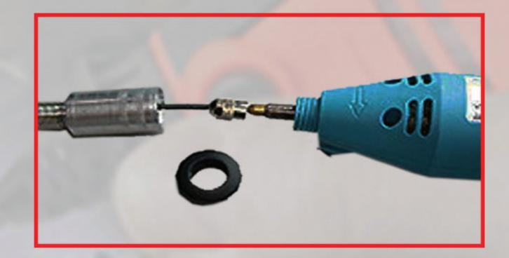
Insert allen key in hole below collet cap to hold spring to change accessories
