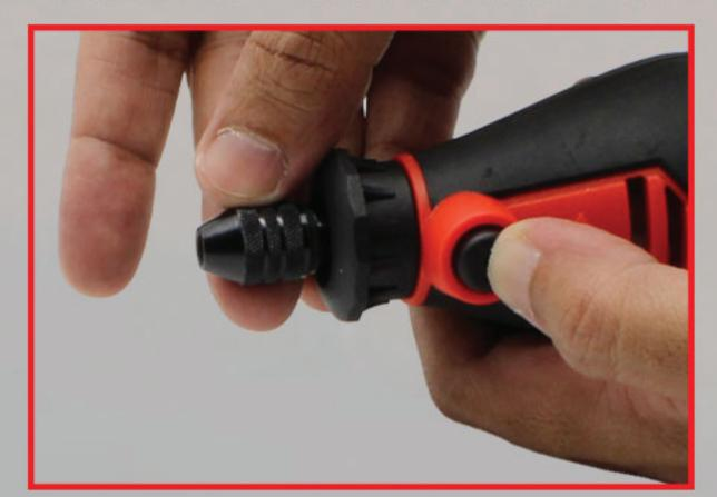
Remove the black collar and insert the inner wire of flexible shaft in universal chuck and tighten it. Tighten the flexible shaft at place of collar
